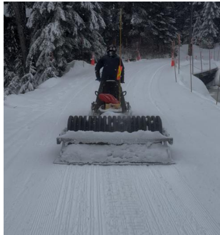
Fig 6: Electric snowmobile with roller in use
