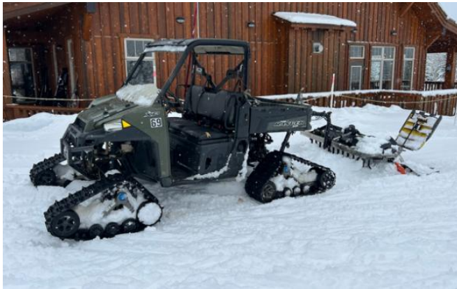
Fig 15: Ginzu groomer with track setting pan pulled by UTV (at another Cross-Country area)
