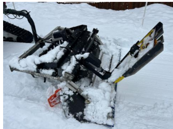
Fig 15: Ginzu groomer with track setting pan pulled by UTV (at another Cross-Country area)
