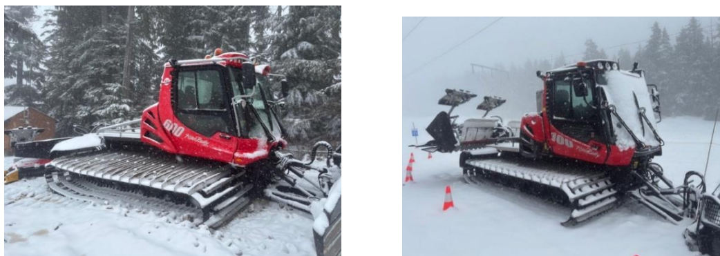
Fig 5: Large grooming machines (PB 600 and PB 100)
